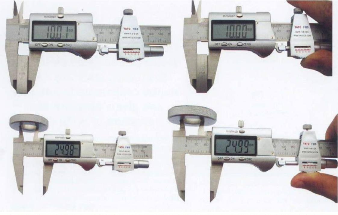
External and internal pressure with a genuine 2-way pressure device. Push or pull. The measurement force used can be seen directly on the device scale.
